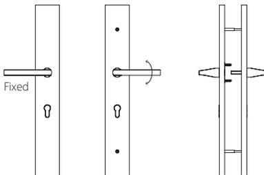
**Dummy Pair with Cylinder Plugs** (for Non-Active Door)
