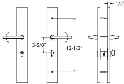
**Non-Keyed with Cylinder Plugs, Passage** (for Semi-Active Door)
