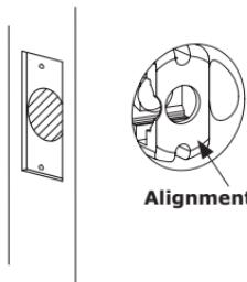
**Step 4B: Insert the latch through the alignment tool.**
