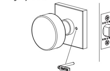
**For emergency, insert Emergency Release Tool into the release hole of the exterior rosette to open the lock.**
