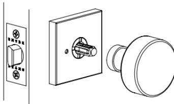
**Step 6D:** Firmly tighten the Pre-installed set screw in the lever or knob with the provided Hex Torque wrench. Ensure that it is firmly tightened.
