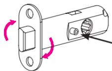
**Privacy Function:** the threaded hole for the privacy pin must be facing the interior side of the door.
