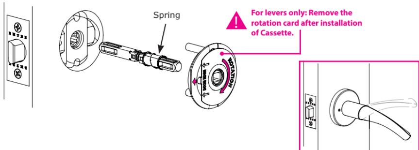
**Step 5B:** Place the CF Cassette B with the arrow pointing to the door edge. Fasten it with (2) machine screws. Check the trim alignment before fully tightening the screws.
