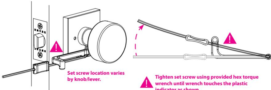
**Step 6E:** Repeat steps 6A-6D for opposite side. For Privacy Lock, screw the Privacy Pin through the rosette, into the latch. To check functionality, turn the interior lever/knob to engage the latch. Now, push the privacy pin in and turn the exterior lever/knob. The exterior lever/knob should not retract the latch.
