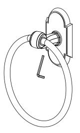
Tighten set screw at base of post with Allen Wrench provided.
