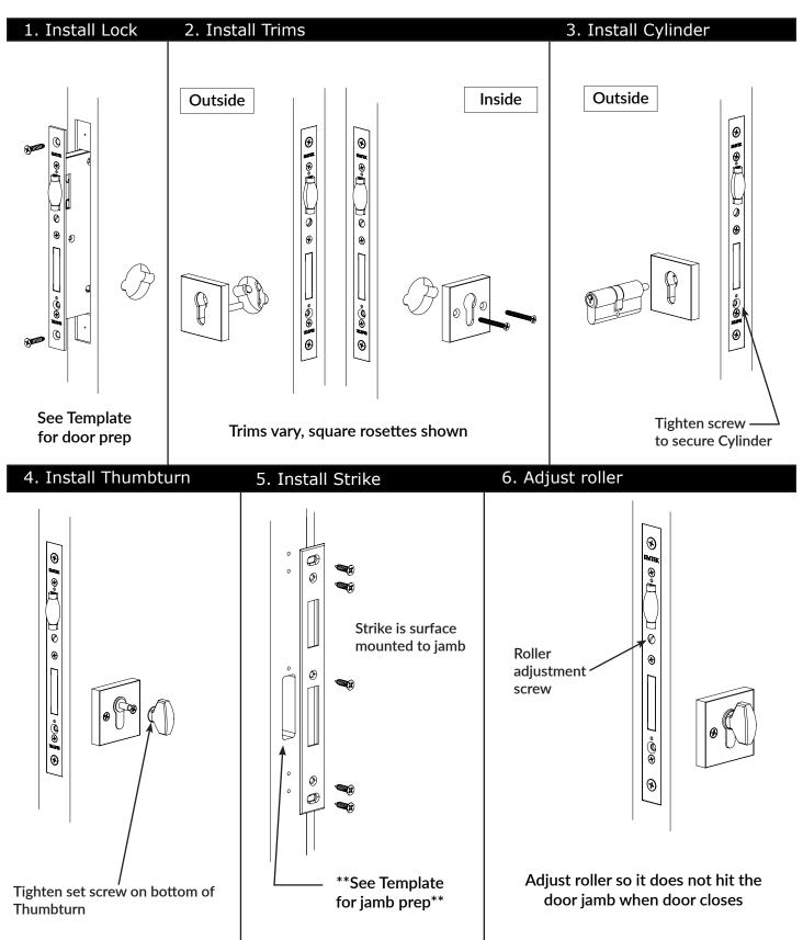
\*\*Only the 5/8" x 2-1/4" rectangle should be mortised in the door jamb. The strike plate should not be mortised as it could impede the function of the roller latch and potentially cause damage to the door jamb.\*\*
