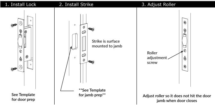
\*\*Only the 3/4" x 1-3/4" rectangle should be mortised in the door jamb. The strike plate should not be mortised as it could impede the function of the roller latch and potentially cause damage to the door jamb.\*\*
