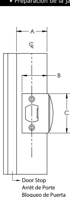
Dimension B & C should be used as reference only. Due to tolerances as reference only. Due to tolerances actual door jamb prep dimensions will vary. Using the strike plate outline edges and locate screw holes on strike with center line on jamb.
