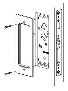
Secure both inside and outside plates using machine screws (provided)
