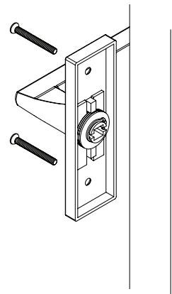
Position trim through the bore holes and tighten with #8 machine screws. (provided)
