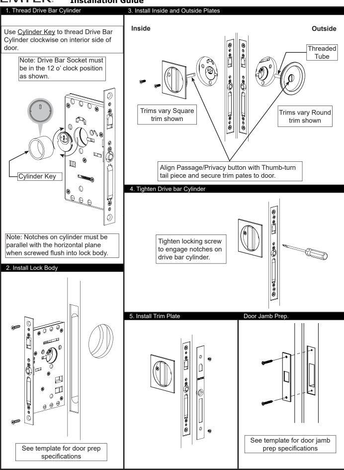
Passage/Dummy Function Installation Guide
