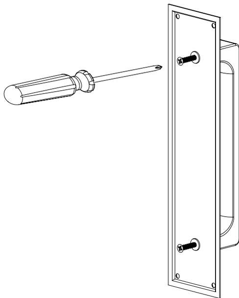
Use #2 Phillips screw driver to fasten plate to handle using #8-32 or 1/4-20 machine screws (provided).
