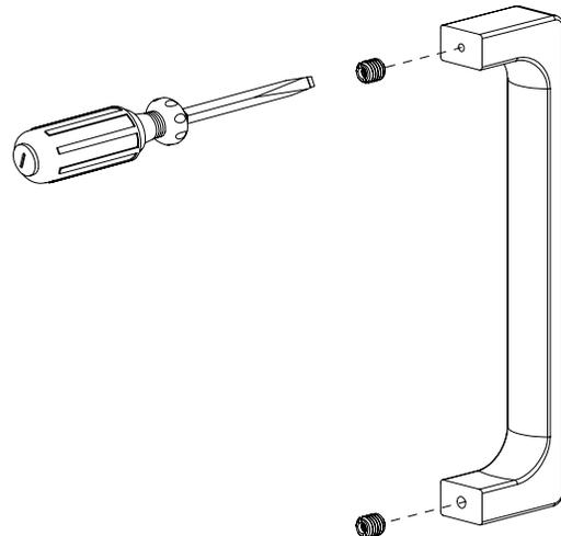
Note: Threaded insert pairs are provided with 8-32 & 1/4-20 internal threads to be used with corresponding screw size.
