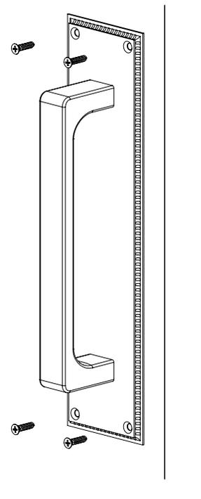
Position Door Pull on door and secure with wood screws (provided).
